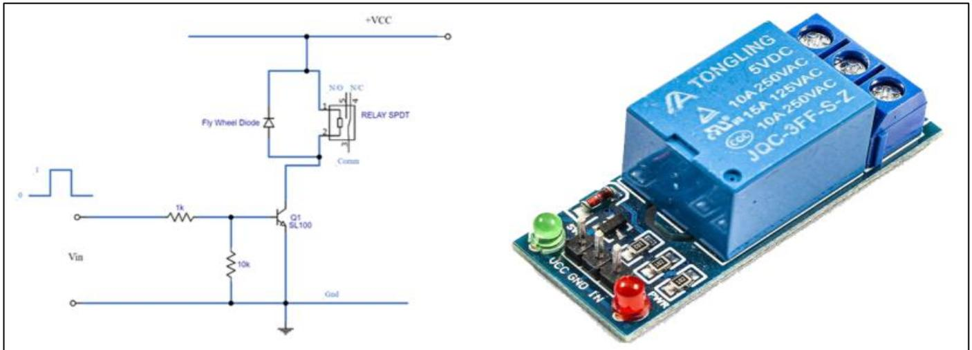
Fig 3 Relay and Relay Driver Circuit
