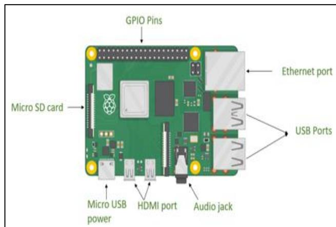
Fig 2 Configuration of Raspberry Pi
