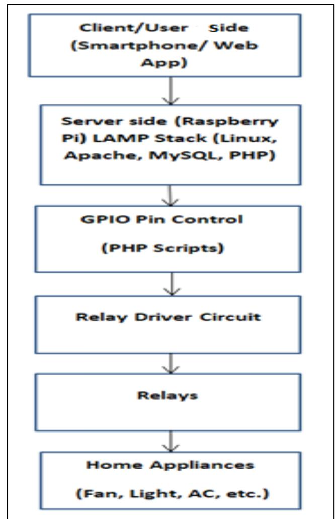
Fig 4 Block Diagram of Proposed Methodology
